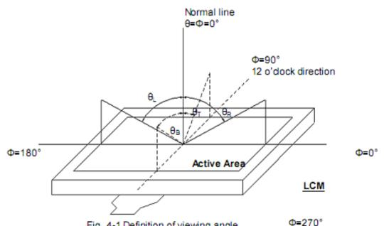
Fig. 4-1 Definition of viewing angle Note 2: Definition of optical measurement system.
