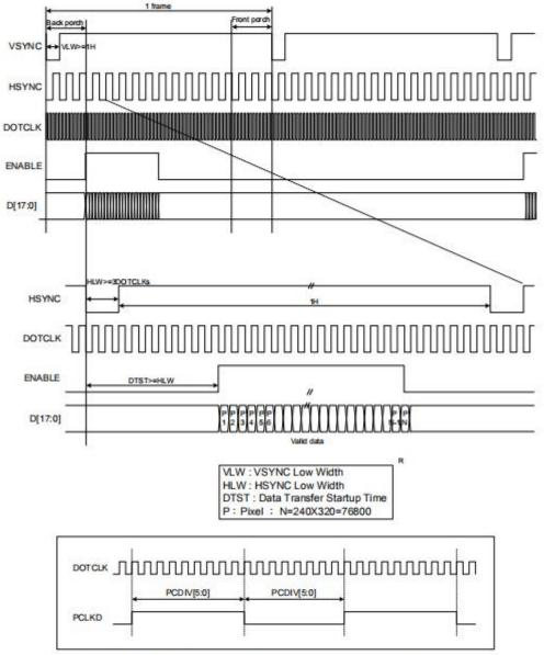
Note 1: The DE signal is not needed when RGB interface SYNC mode is selected. Note 2: VSPL='0', HSPL='0', DPL='0' and EPL='0' of "Interface Mode Control (B0h)" command.
