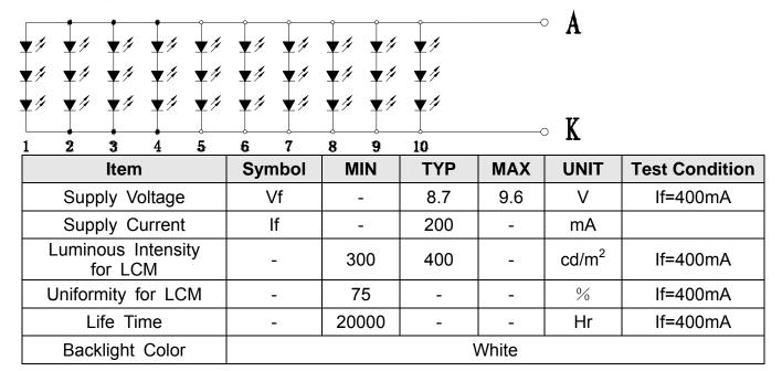
Note 1: The LED Supply Voltage is defined by the number of LED at Ta=25 $^{\circ}$ C and IL = 400mA.
