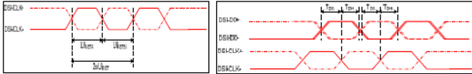
Figure 4 DSI clock channel timing
